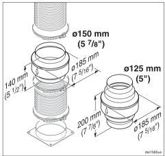
In some cases, a condensate trap may also be required to collect and evaporate any condensation which may occur. This optional accessory is available for ducts 5" (125 mm) and  $5^7/_8$ " (150 mm) in diameter.
